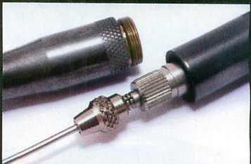
Classic needle-chuck design lies beneath the handle.
