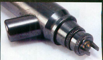
The crown features a two-pronged design for a clear view of the needle.
